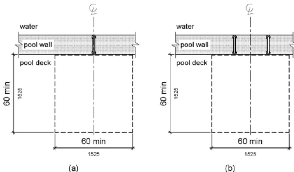
**Figure 1009.4.1 Clear Deck Space at Transfer Walls**
