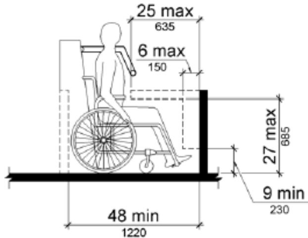
**Figure 1002.4.4.3 Protrusions in Wheelchair Spaces in Amusement Rides**
